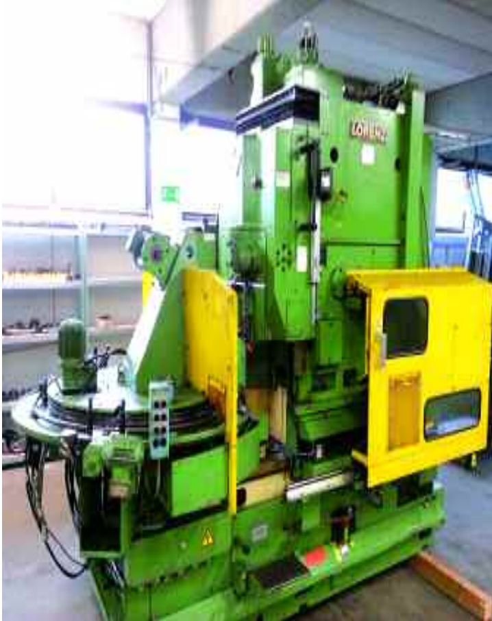
LORENZ LS 180 CNC 1984 Wälzstoßmaschine Ø 280 x Mod. 4 CNC gear shaper with ring loader
