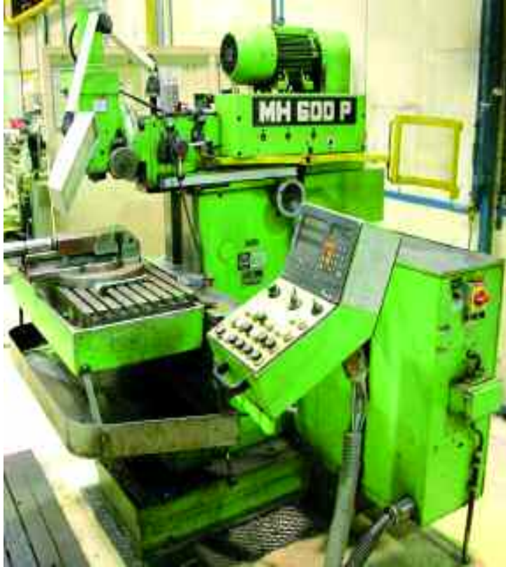
MAHO MH 600 P Universalfräsmaschine 500 x 400 x 400 universal milling machine + Heidenhain
