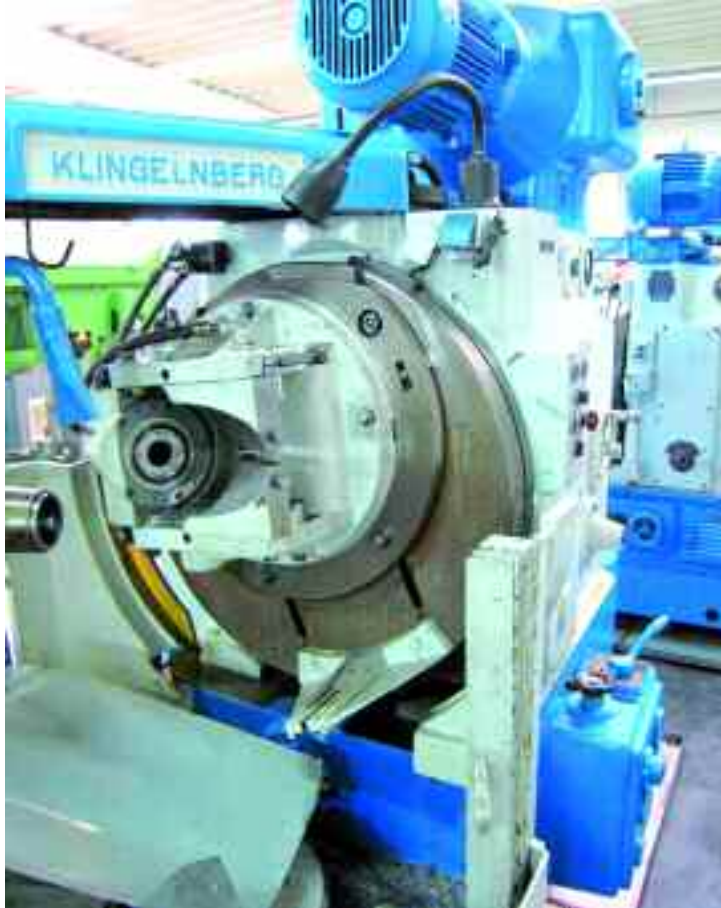
KLINGELNBERG AFK 201 1965 Palliod-Kegelradfräsm. Ø 540 mm x Mod. 8 bevel gear generator, gear width 275 mm
