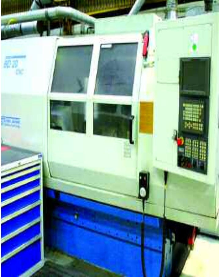
JUNKER BD 20 CNC 2000 CNC-Innenschleifmaschine CNC internal grinder
